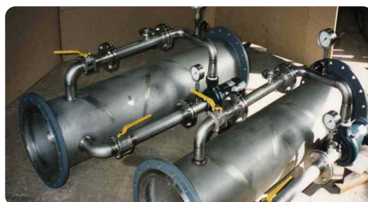
Reliable solubility of the CO 2 gas thanks to special design of the static mixer
