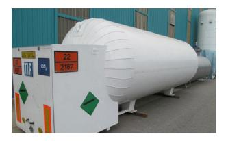
**ASCO** supplies different sizes of transportable  $CO_2$  tanks which can be mounted on any suitable truck or trailer locally. Transportable tanks are a cost saving alternative to conventional road tankers as the operator may use the vehicle for other duties as well as bulk  $CO_2$  transport. The tank is a self-contained unit mounted on a base frame and when empty it can easily be craned on or off as required. Suitable lifting lugs are on the top of the tank.
