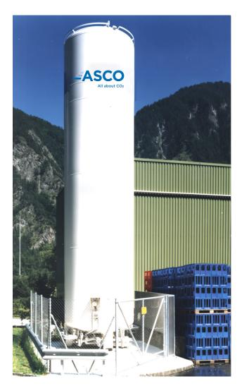
**ASCO**  $CO_2$  Storage Tanks include a high quality perlite vacuum insulation and are supplied complete with all pipework, valves, safety devices, liquid level indicator, pressure gauge, automatic pressure build up and pressure reducing systems allowing fast and easy installation on site.
