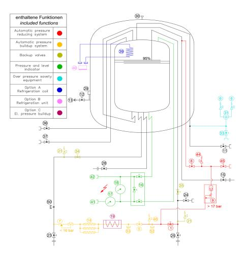
All pipework is aligned inside the tank and the connections are at the bottom of the tank.
