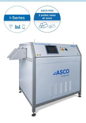
The **ASCO** Dry Ice Pelletizer P55i is one of the most powerful dry Ice machines from **ASCO**'s i-Series line. Having a production capacity of 550 kg/h (1212 lb/h) it meets the demands for high dry ice quantities plus quality and flexibility in the daily working process.
