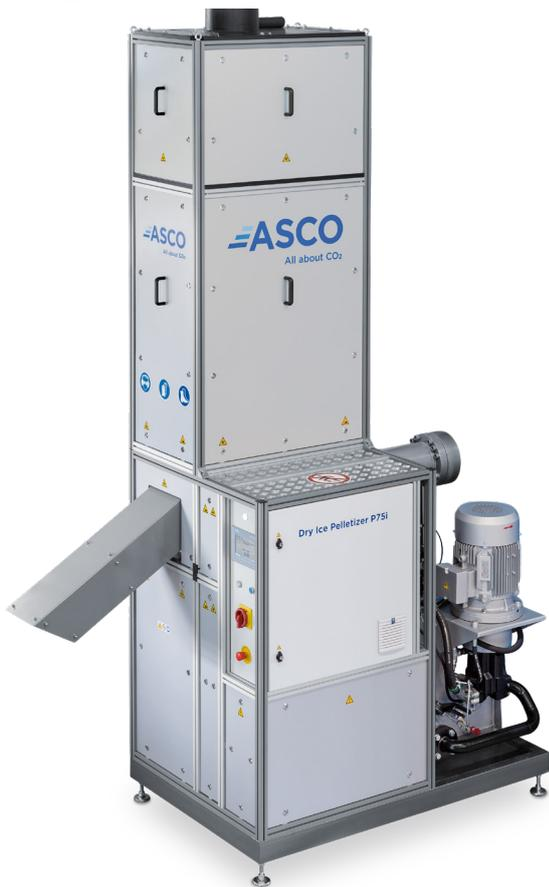
The Pelletizer P75i is the most powerful model in the range of **ASCO i-Series dry ice production machines**. At ASCO, i-Series stands for interconnected production. Be it for quick and efficient trouble shooting and maintenance or for gathering of production and performance data - the i-Series offers a wide range of options to link industry 4.0 dry ice production to industry 4.0.
