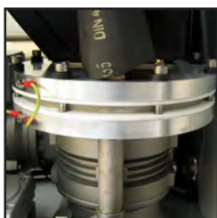
Distributor unit for pulsation-free blasting
