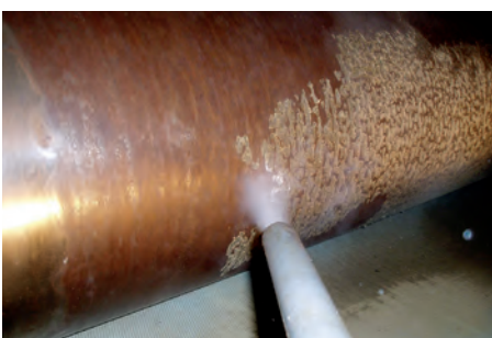
Dry ice cleaning in the paper industry: The removal of paper residues and lubrication oil from paper production machines also eliminates burn marks.
