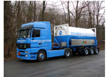
ISO container for transportation of CO 2
