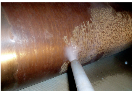
Dry ice cleaning in the paper industry: The removal of paper residues and lubrication oil from paper production machines also eliminates burn marks.
