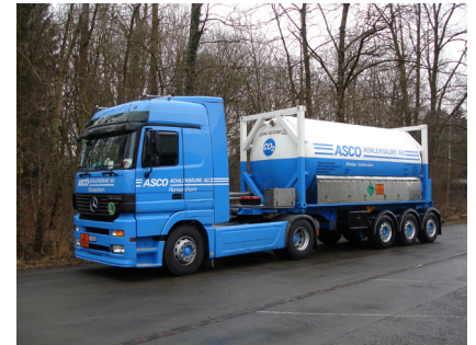
ISO container for transportation of CO 2
