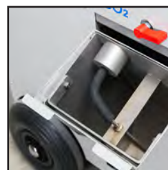
Box for additive with approx. 12 kg (26 lb) capacity
