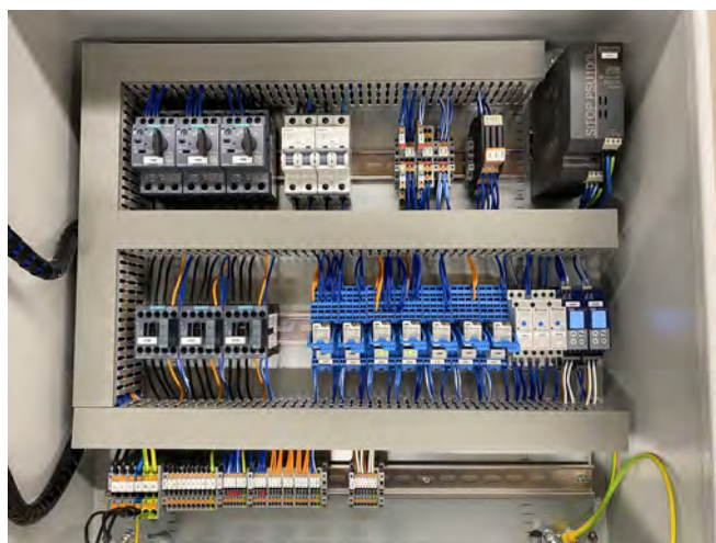
External control cabinet with 10 m connecting cable, temperature sensors and cabinet heating
