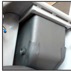
Insulated pellet hopper with 9 kg (20 lb) capacity
