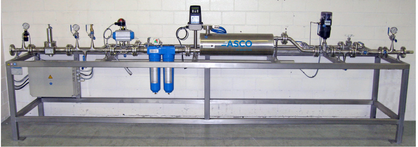
ASCO CO 2 Dosing System (single line)
