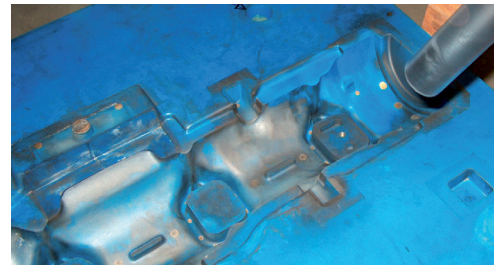
Core box cleaning in a grey iron foundry
