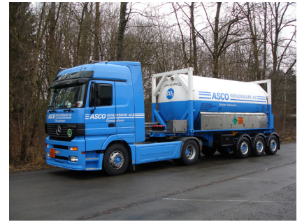
ISO container for transportation of CO 2
