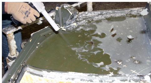
Cleaning of a mould in PU-production
