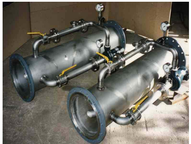
Reliable solubility of the CO 2 gas thanks to special design of the static mixer
