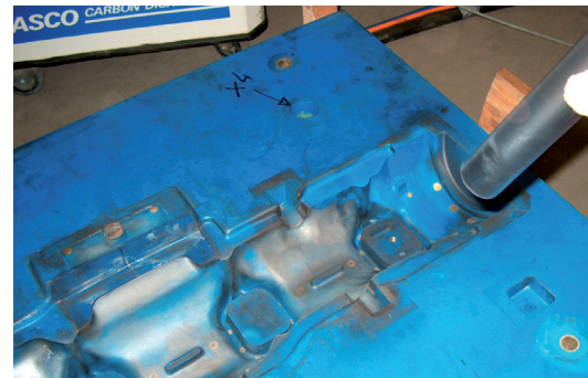
Core box cleaning in a grey cast iron foundry
