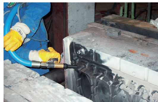
Cleaning of built-in hot ingot moulds
