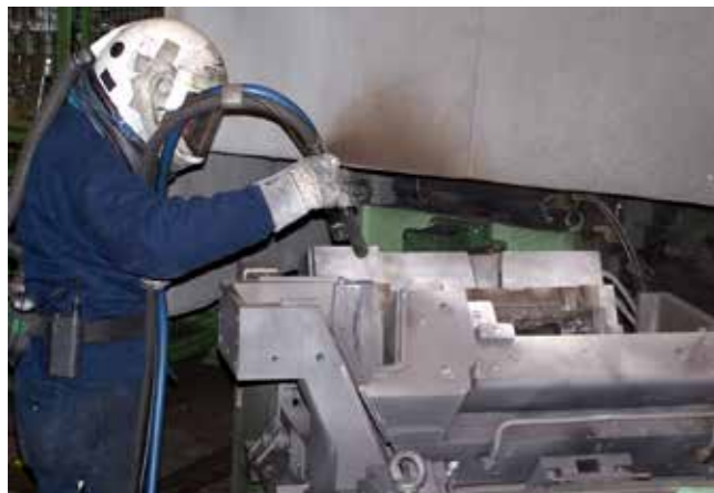
The mould cleaning is perfectly integrated in Daimler's working process.
