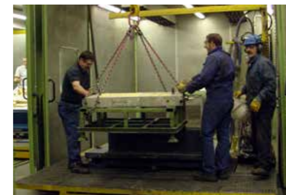
The core boxes are prepared for cleaning in a noise control booth.
