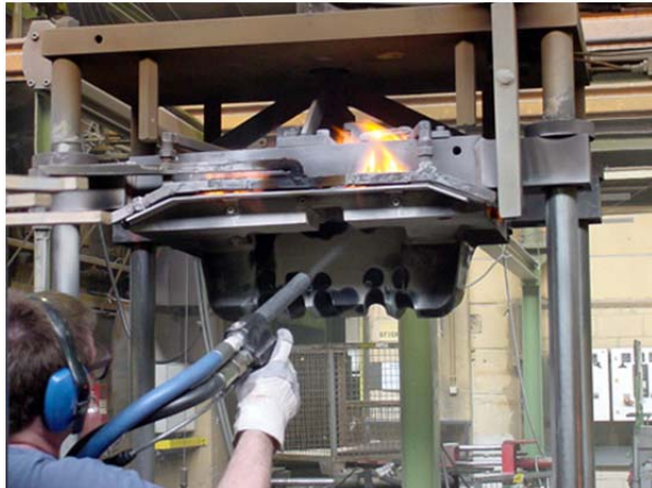
Efficient online cleaning of a hot ingot mould.
