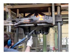
Efficient online cleaning of a hot ingot mould.
