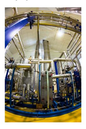
Pictured: Process unit with heat exchangers and pumps in the front, absorber and desorption columns in the background.
