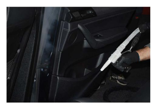
Dry ice blasting can be used perfectly for cleaning of vehicle interior.
