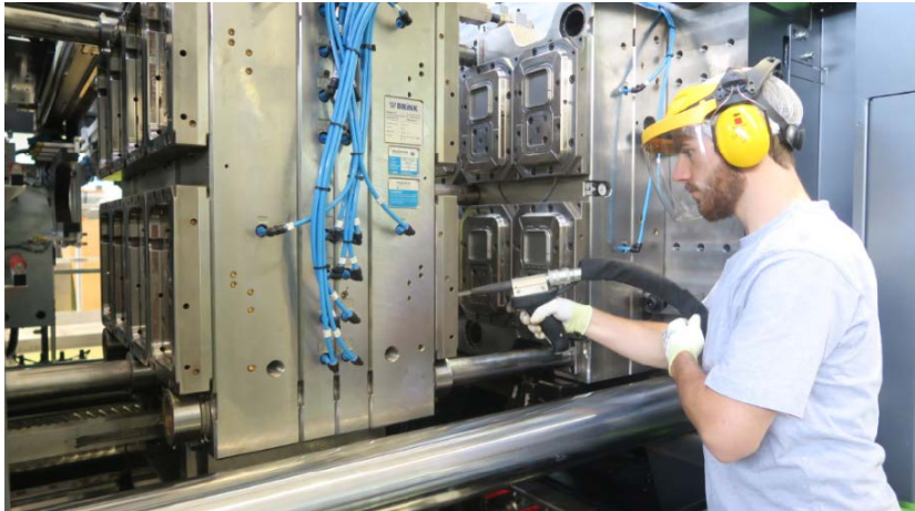
Figure 1 – Cleaning of moulds with ASCO dry ice blasting technology
