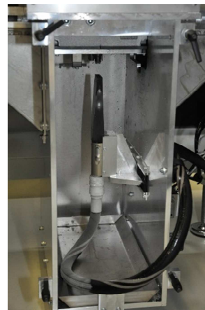
Picture 2: Blasting nozzle integrated into the production line
