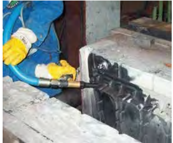
Fig.3: Online cleaning of a hot mold
