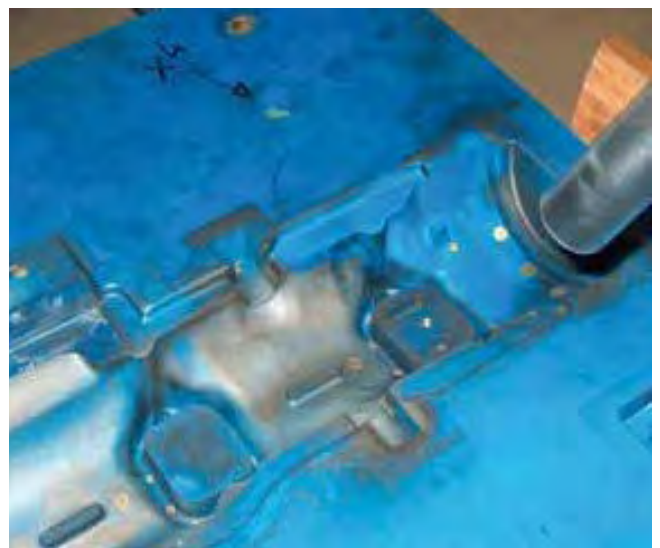
Fig.2: Core box cleaning in a grey cast iron foundry
