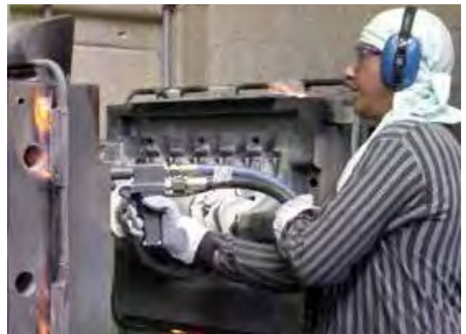
Fig. 6: Cleaning of built-in hot molds
