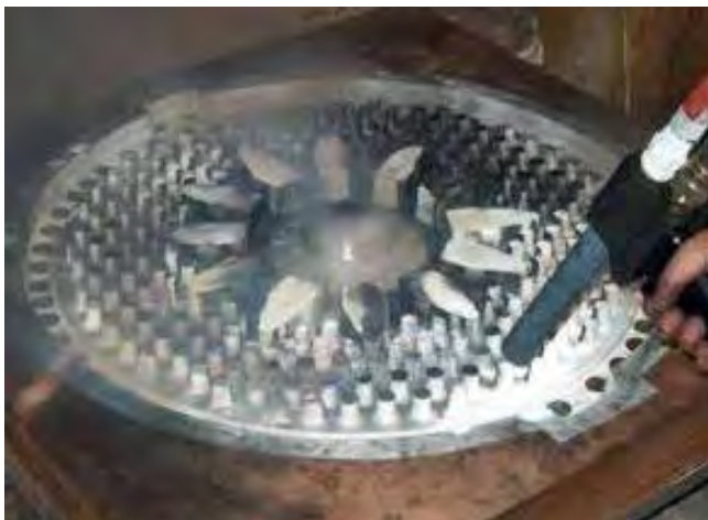
Fig. 5: Cleaning of a core box in the automotive industry
