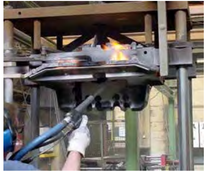
Fig. 7: Removal of release agent from a PU core box
