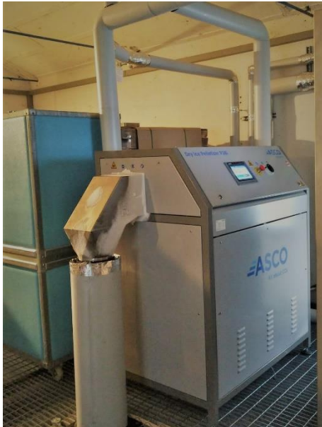
Dry Ice Production Machine ASCO P28i
