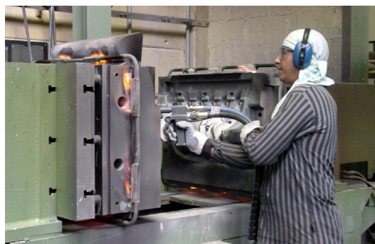
Cleaning of a built-in, hot mould
