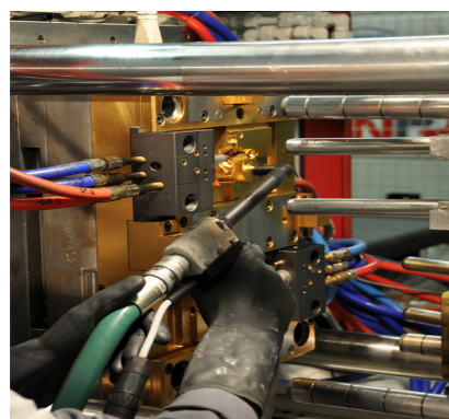
Cleaning of a built-in, hot mould
